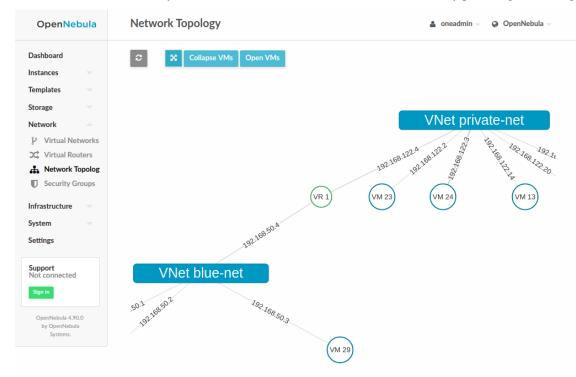
The Virtual Networks connected to the VR machines can be modified with the attach/detach actions.
